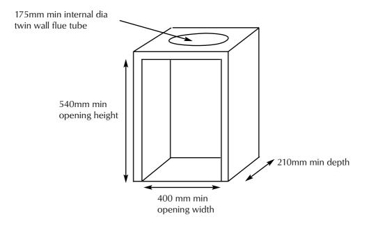
Some flue boxes may require minor adaption when fitting the fire using the cable fixing kit. The firebox, base of the flue box, and the hearth may be drilled to allow plugs and screws to secure installation.
