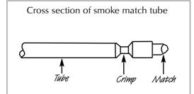
Make a smoke match tube from 10mm diameter tube. Seal off one end and crimp the tube to prevent the smoke match from sliding down inside.
