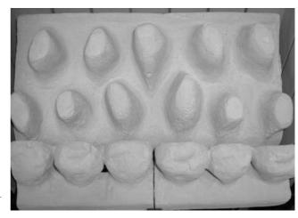
2. Open the bag of 22 ceramic pebbles. All of these pebbles are the same size. Take five pebbles and place them as shown. Care should be taken to ensure that the pebbles bridge the gap between the front strip and the six supports at the front of the matrix. Care should also be taken not to push the pebbles right down between the supports, as this can affect the flame picture when the appliance is running.
