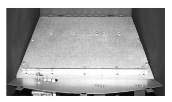
If the data/control plate is not already fitted, attach with two screws, ensuring the control knob is free to be depressed fully.
