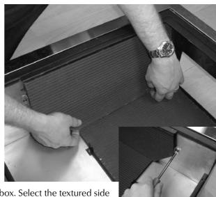
The three radiant panels may now be fixed inside the firebox. Select the textured side of each panel and insert as follows; Lay the firebox on it's back. Lay the large rectan-
