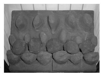
4. Take five more moulded coals and position as shown to form the 'second row' of the fuel effect. The coals may be rotated as desired to fit into the gaps between the coal supports in order to create a random, realistic effect. Again, remember not to push the coals down too far into the valleys between the coal supports as this can have a detrimental effect to the flame picture.
