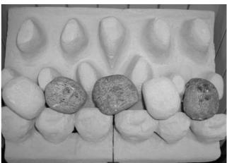
3. Take five more ceramic pebbles and position as shown to form the 'second row' of the fuel effect. The pebbles may be rotated as desired to fit into the gaps between the supports in order to create a random, realistic effect. Again, remember not to push the pebbles down too far into the valleys between the supports as this can have a detrimental effect to the flame picture.
